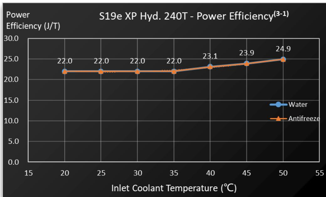
(3-1) The hashrate value, and power efficiency on wall are all typical values. The actual hashrate value fluctuates by  $\pm 3\%$ , and the actual power efficiency on wall fluctuate by  $\pm 5\%$ .
